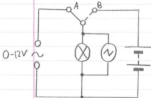
The D.C. Voltage was measured with a voltmeter. The peak A.C voltage was measured with an oscilloscope in position A.
