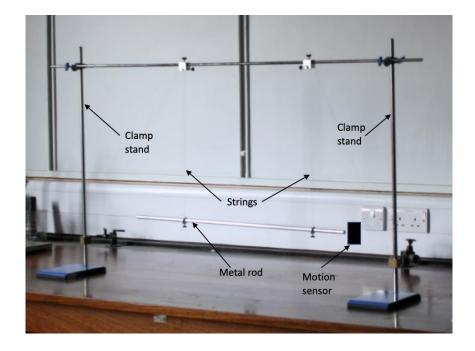
A metal rod was first measured, and the midpoint found and marked. This midpoint was then used to mark lines at every 5cm intervals starting at a 10cm radius. Then the rod was hung by strings that we both tight but easily loosened and adjusted. In this way, the string was placed at the first mark on the rod at 10cm. A light or motion senor was placed at the end of the pendulum so that it could track the swings as the pendulum moved. A torch was used to make this easier.
