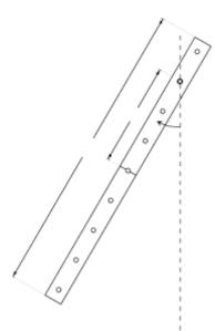
The restoring torque for an angular displacement  $\theta$  is:  $\tau$  = - mg l sin $\theta$ Where l is the distance to the centre of mass
