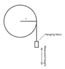
The mass and radius of the wheel being used were measured. Attach a mass hanger to a piece of thread and then connect this to the wheel and then measure the height the mass will be dropped from. Add small masses to the hanger until the mass falls with a uniform velocity. Wind the thread around the wheel until the test mass is at the correct height and then release the mass and time the descent. Record the value of the mass being dropped and repeat the experiment 5 times for each mass.
