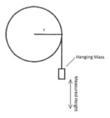
The mass and the radius of the wheel being used were measured. Attach a mass hanger to a piece of thread and then connect this to the wheel and then measure the height the mass will be dropped from. Add small masses to the hanger until the mass falls with a uniform velocity. Wind the thread around the wheel until the test mass is at the correct height and then release the mass and time the descent. Record the value of the mass being dropped and repeat the experiment 5 times for each mass.
