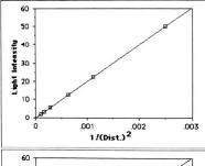
By plotting the reciprocals of the distances squared versus the intensities, we now have a straight line graph. This is a solid indication of the type of proportion that is at work in this lab.
