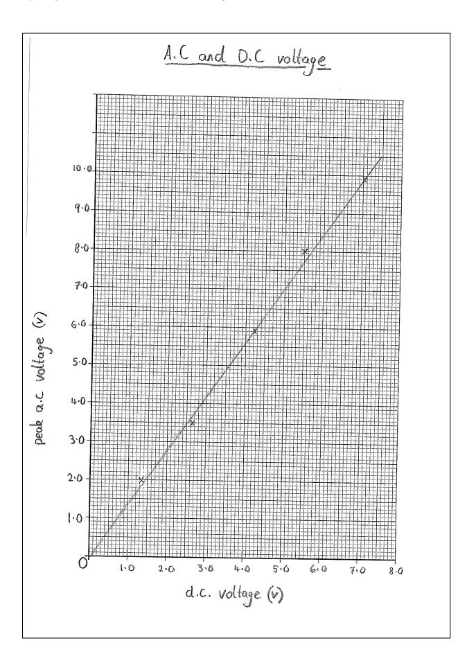
A.C and D.C voltage Analysis (5.0,7.0) (2.5,3.5)  $m = \frac{y_2 \cdot y_1}{2c_2 - 3c_1}$ The gradient of the graph plotted is 1.4 which shows that the peak a.c. voltage is = 7.0-3.5 5.0-2.5 = 1.4 a factor of 1.4 higher "than its d.c equivalent. Second Source Reference 1 Vm (volts) Vac (volts) 8.5 12.0 lamp 1 3.0 2.1 lamp 2 2.0 1.4 lamp 3  $V_{m} = 12.0$  $V_m = 3.0$  $V_m = 2.0$ Vdc 2.1 8.5 1.4 Vdr Velle = 1.4 = 1.4 = 1.4
